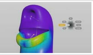
Select the *jointcapturepaint* node. Click on the pull down menu in the **Capture Region** field and choose the *jaw* joint. **Press F** and choose **Subtract** to take away influence of this joint on the top of the head and eye area.
