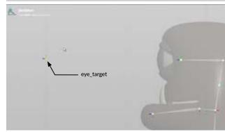
Pan to the area around the eye. Go back to **Create** model and **MMB-click** to any connections. Now add a new joint out in front of the eye.
