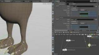
Select the rigpose\_feet node. Make sure only the left and right ball and toe joints are listed on this node. For all of them, RMB-click > Lock Parameter on the Translate, Rotate and Scale parameters. Then go to the Rotate Y for each of them and RMB-click > Unlock Parameter.
