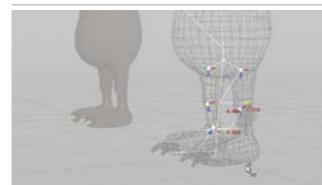
Add a **Rig Pose** node in-between the *parent* node and the *ikchains* node. Click on the *ankle* joints and move them around to see the Inverse Kinematics at work. Because you used **Match by Name** the ankle joints are acting as the end effectors for the IK chain.
