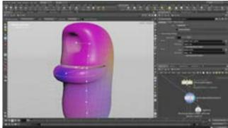
Set the **Display Flag** on *jointcapturebiharmonic*. Now **bypass** the *add\_capture\_geometry* node to show difference in the capture weights.
